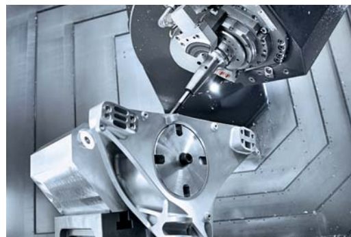
With highly precise and productive 5-axis machining, toolcraft produces complex precision parts (example: wheel support).
