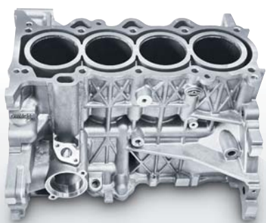
Cylinder block, machined on a DMC 80 H linear
