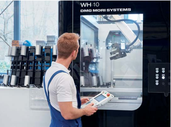
The NLX 2500 handling system is designed for max. 26.5 lbs. workpieces
