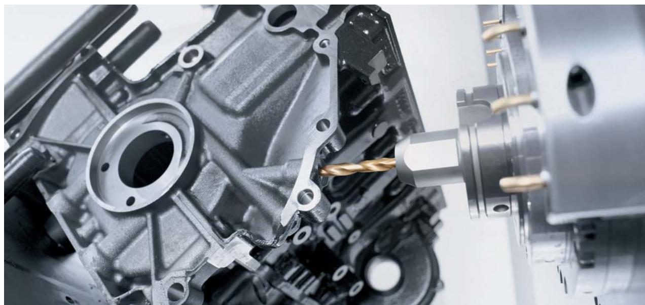
Swivel rotary table with a swivel angle of 225° – highly productive 5-axis machining in one setup.
