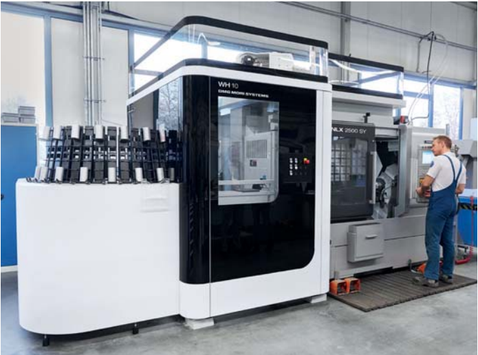
To increase capacity and productivity, Maske recently invested in a NLX 2500 with WH 10 top workpiece handling.
