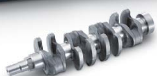
\varnothing 7.9 \times 39.4 in. Crankshaft / Automotive Material: S45C Production time: 40 min.
