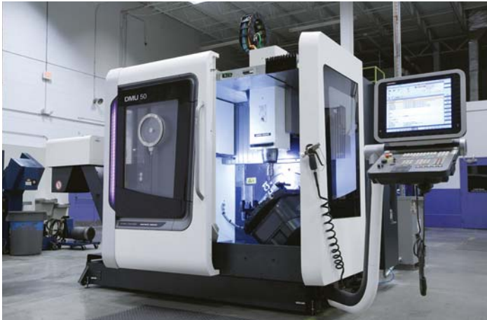
Sparton recently purchased a DMU 50 5-axis CNC universal milling machine to stay ahead of the competition and grow into new markets
