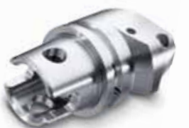
6-sided complete machining with main and counter spindle; maximum productivity through use of 2 tool holders.
