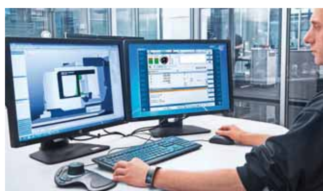
The DMG MORI Virtual Machine is a 1:1 mirror of the DMC 160 H duoBLOCK® including the actual control unit.
