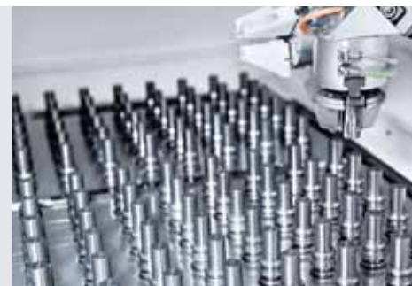
Thanks to integrated automation, M.T. produces lot sizes of up to 1,500 parts almost entirely on unmanned systems.
