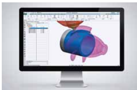
Hybrid CAD / CAM for additive buildup and chip removal.
