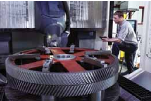
DMU 210 P and gearMILL® Software for complex machining of an AGMA Q11 herringbone.
