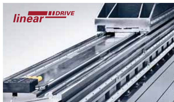
Above: DMU 600 G linear being set up at the XXL-Centre of DECKEL MAHO in Pfronten, the world's most modern large machine production facility. Below: Consistently high precision due to temperature stability of machine structure.
