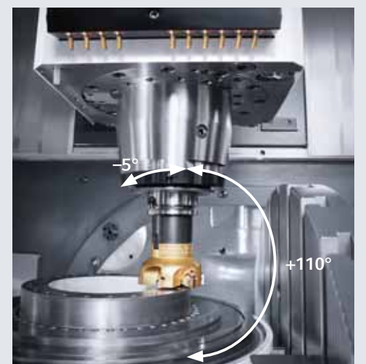
Swivel range of NC rotary table: -5° to +110°.
