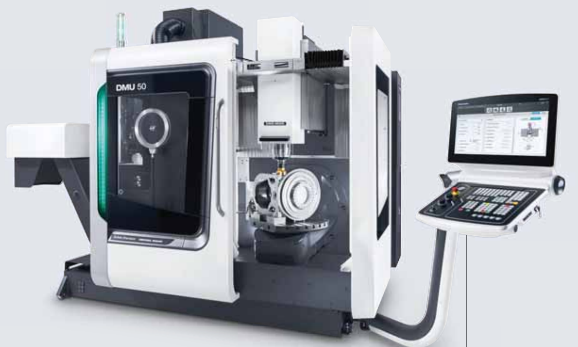
Swivel range of NC rotary table: -5° to +110°.
