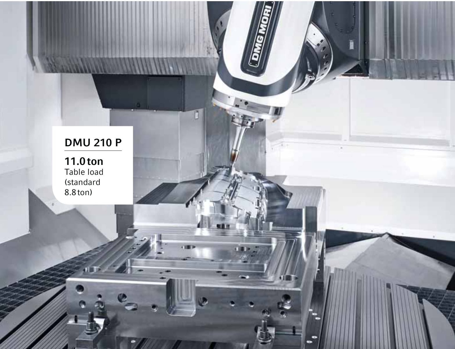
DMU 210 P and gearMILL® Software for complex machining of an AGMA Q11 herringbone.
