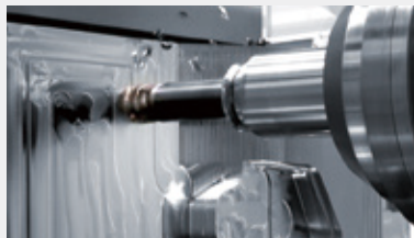
Profiling (mold) Highly efficient rough machining of highly tough material (40HRC) \phi 63 [ \phi 2.5 in.] high feed cutter
