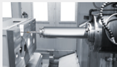
W-axis (boring spindle) feed machining
