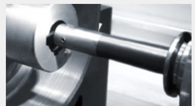
Cs control slotter machining 13-square high-speed steel tool Material: FCD
