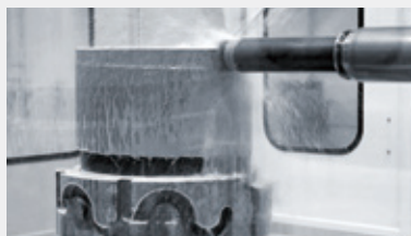
Continuous rotary machining Rotary cutting by rotating the rotary table is enabled as standard
