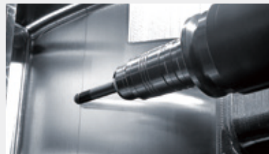
Profiling (mold) Semi-finishing of highly tough material (40HRC) \phi 16 [ \phi 0.6 in.] ball end mill
