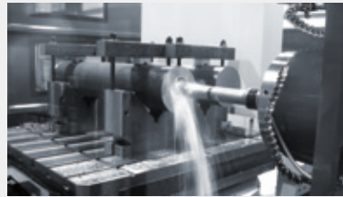
Deep-hole drilling \phi 110 mm [ \phi 4.3 in.] fullcut drill / Material: S55C
