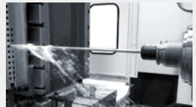
MC gun drilling \phi 16 [ \phi 0.6 in.] machine gun drill / drilling depth: 800 mm (31.5 in.)
