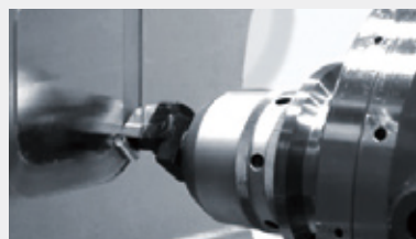
Cs control spring neck machining Carbide tool Material: SUS3040
